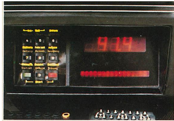
Left: centre console shows time in this shot. Nine functions can be monitored and displayed
