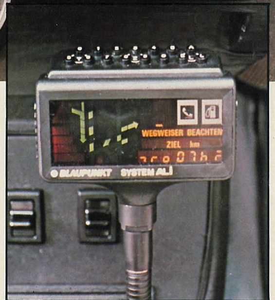
Above: nose air-dam and flared arches hint at a rather different temperament... Right: Blaupunkt's ALI route guide display in what b+b calls 'modest black and white'
