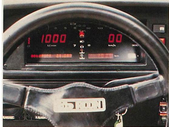
Left: main instrument panel is all-digital here showing 1,000 rpm at 0 mph
