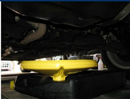
Place your oil drain pan under the oil pan drain plug.
