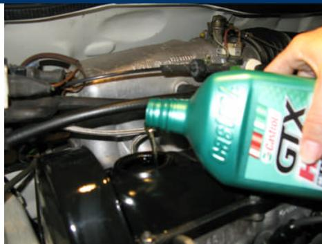
Remove the oil cap on the valve cover and refill the crankcase with new oil (use a funnel if desired), checking the dipstick as you go once you have added 3.5 - 4 quarts. Stop filling once the level is in the middle of the dipstick indicator.
