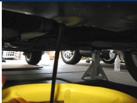
Loosen the oil pan drain plug using your preferred 19mm wrench; remove the drain plug by hand. Allow the oil to drain until it becomes a slow drip.
