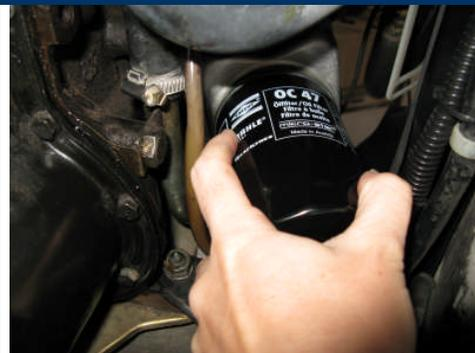
After wiping the filter flange clean, install the new oil filter by hand. Screw the filter into place until the gasket contacts the flange, then turn the filter another  $\frac{3}{4}$  turn to tighten it.
