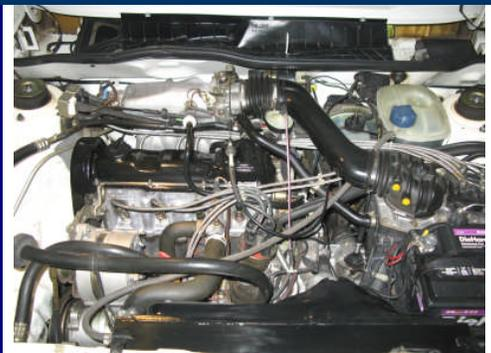
Replace the oil cap on the valve cover (wipe the cap and the valve cover opening clean, first) and run the engine. After about 3 minutes, turn off the engine and check for oil leaks.
