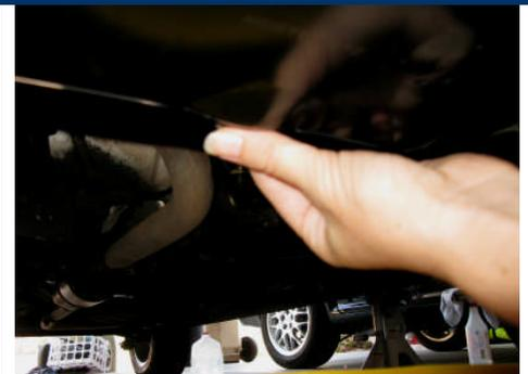
Wipe the drain hole clean and reinstall the drain plug using a new metal sealing washer. Screw it in by hand as far as you can; then, using your torque wrench with 19mm socket, torque the drain plug to 30Nm (22 ft. lb.).
