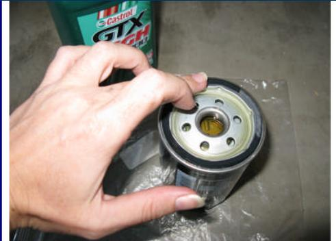
Add a bit of new oil to the new filter. Do not overfill the filter; if oil touches the threads, there's too much. Lightly lubricate the new filter's gasket with fresh oil.
