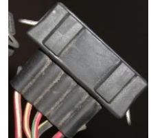
2-pin at each injector; 5-pin at end of fuel rail
