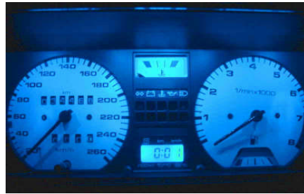
blue LEDs (not installed in original bulb locations)
