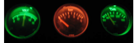
green LEDs (center is stock bulb)
