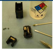
Once the contact is working right, give the entire switch a good cleaning out of the 25 years or so of built-up crud inside. Alcohol and Q-tips work great for this. Especially clean and inspect the base contacts for severe wear. A new switch is warranted if they're too far gone. (Yep, mine was pretty crusty.)
