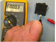
Test the switch to see if it works and that you bent the contacts enough. The meter should read infinite when the switch is off and less than an ohm when the switch is on. If not, go back in and bend/clean the contact a little more.
