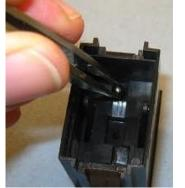
Reassemble. Remember the little metal ball? It goes back in the switch as pictured, at the indent at one end.
