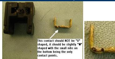
You're mostly concerned with the "spring loaded contact" component. Remove the Ushaped contact. It should slip right out. Be careful of the spring underneath it and the spring on the opposite side that pushes on the little metal ball. Both of these springs should sit freely in the hole, not binding. If either spring binds, or is damaged, you found your problem. Replace.
