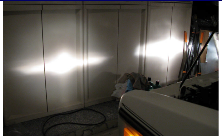
Lo-beams, after 13.36 VDC
