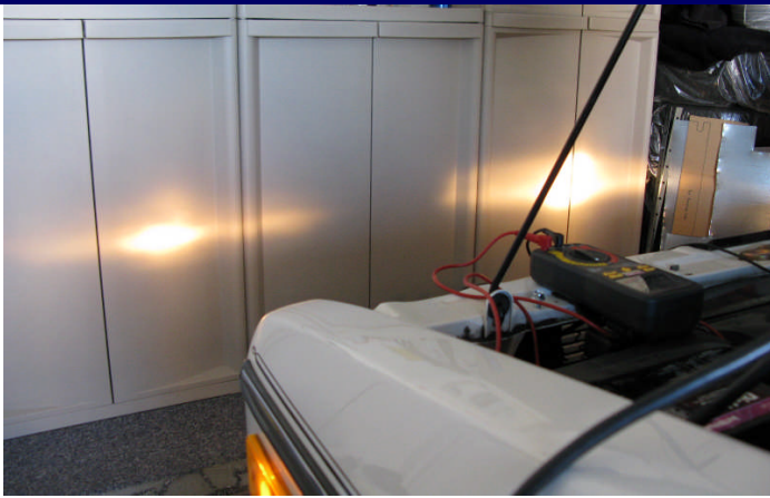
Lo-beams, before 10.68 VDC
