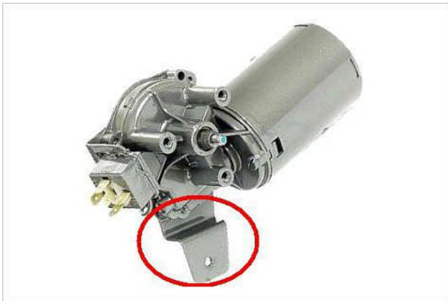
This is the back plate from a Mk3. Notice the lack of bracket.
