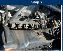
Remove the accelerator cable, ISV\* and vacuum hose going to the brake servo; this will give you more room to work.
