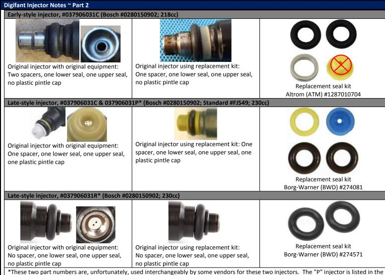
\*These two part numbers are, unfortunately, used interchangeably by some vendors for these two injectors. The "P" injector is listed in the official Volkswagen parts catalog for the 2H engine as the direct replacement for the "C" injector, and is the recommended replacement. The "R" injector is listed by Volkswagen dealers as an equivalent replacement for both "C" and "P" injectors and should work in your 2H without issue.
