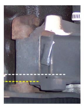
Here it is all put back together. Note the V-belt is not perfectly aligned, but with the addition of a 16mm hole washer behind the pulley it's darn close. I've had it revved out to over 100 with no issues.
