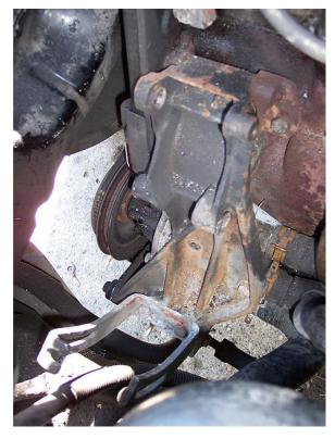
Remove the bolts that hold the big bracket on. There are two bolts that go thru the water pump (13mm) and one long Allen head (6mm) bolt at the top and may only be accessible by taking off the upper timing cover.
