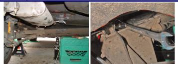
It moved! I kept turning it until I noticed that the whole bushing housing was turning with the bolt and that it had stretched and kinked the parking brake cable. I tucked the cable out of the way with a tie wrap and kept turning until I got the nut loose. Dropped the beam a bit more and I was able to remove the whole bushing/housing/bolt assembly with just a bit of hammer/punch persuasion.
