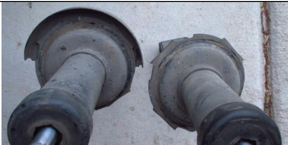
Example of what needs replacing: Original, 29-year-old rear shocks with busted spring seats
