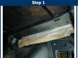
Open the boot (trunk). Look up and find the tabs that the headliner is secured with. Pull the headliner off the tabs and let it hang there.
