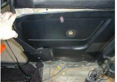
Remove the window knob by prying up the cover and unscrewing it. This is in the Haynes and Bentley. Remove the interior card by pulling the door trim away from the edge and prying the fasteners loose. They will pop out. The seat belt trim may have a little holding knockout that will have to be pried up.
