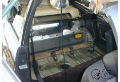
Remove the rear seatback by unscrewing the two screws at the base of it. Open your boot and pull the release button, and then the release cord. This is a bit of a maneuver, but by lifting and pulling, the seatback will come out. Set it aside.
