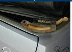
The removed headliner fitting is here. Note the plastic rod that is in the headliner tab.
