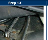
Next step could be done before, but I didn't think about it. Duh. You now have to free the window frame hinges and the rear headliner tabs. Pull the top up at the back and look for the hinge mounts. Each has two bolts. Remove the bolts. The itty bitty wrench is your friend for the bottom one. If you did this while the top was still on the car, you could probably reach both with a socket.
