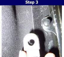
Pull the strut's upper-end off of its mounting post.
