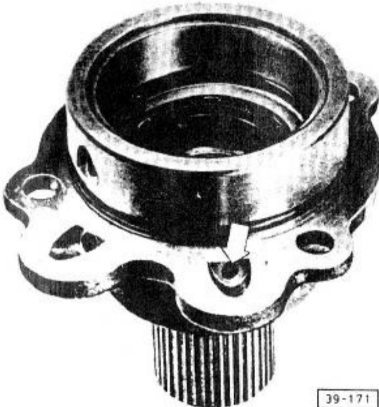
Fig. 18 One-way clutch support, checking ball valve
