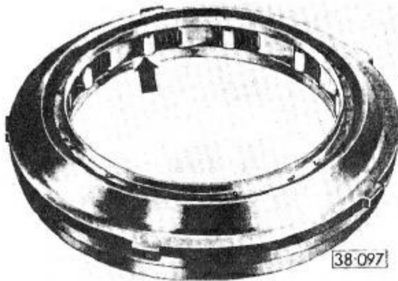
Fig. 7 One-way clutch / spacer springs and rollers, assembling — rollers must be assembled in cage as shown (arrow)
