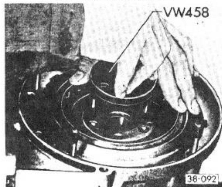
Fig. 9 One-way clutch, installing and checking — clutch can also be turned with tool as shown — checking: it must not be possible to turn planetary gear set counterclockwise
