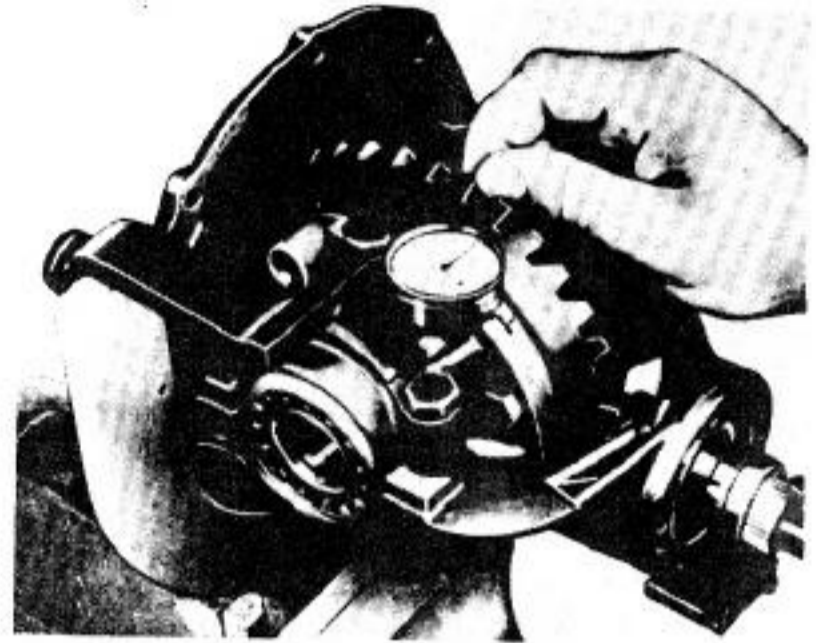
Fig. 11-35. Measuring backlash. The dial indicates the amount of ring gear rotation.
