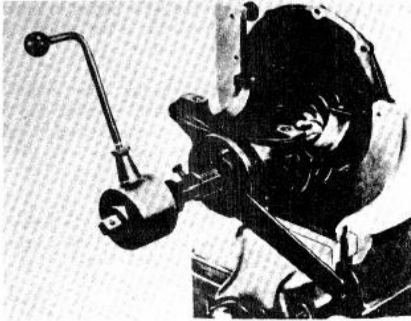
Fig. 11-28. Pinion and carrier in vise for preload measurement.
