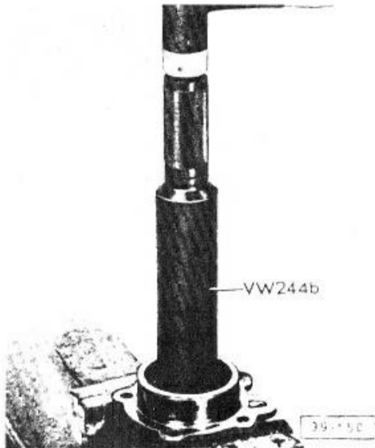
Fig. 11 Oil seal/pinion shaft, installing – sealing lip toward converter
