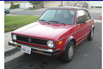
Claimed car year: 1989 Incorrect parts: wheels, bumpers, headlight grille, fender flares (car resembles an '86/'87)
