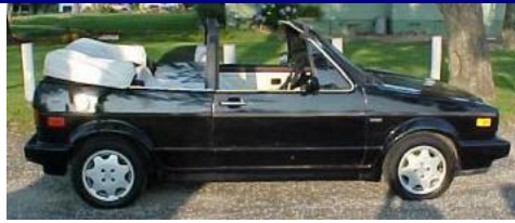
Claimed car year: 1987 Incorrect parts: Clipper kit, interior, and 1991+ wheels (car received a complete make-over)
