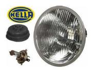
A 7" round headlamp and dual-filament bulb assembly that looks like a sealed-beam headlamp that uses a replaceable H4 or 9003/HB2 bulb. The H4s came standard on European cars (see E-code below). The 9003/HB2 is the DOT's version of the H4, but these were never installed on the cars at the factory. The two bulb types are slightly different: the H4 is designed for E-codes, while the 9003/HB2 bulbs are designed for DOT. All, however, use the same socket pattern.
