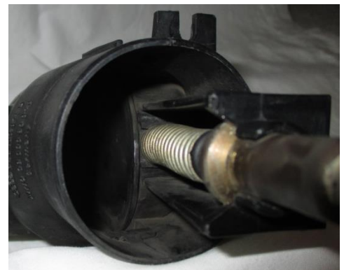
Sensor warm; flap closed to warm air
