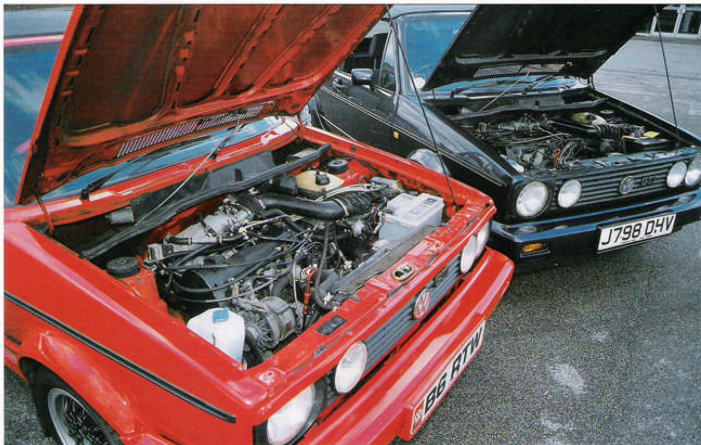
Most late model Cabrios feature the classic fuel-injected 'DX' engine, but be very wary of the less powerful catalyst-equipped 'JH' unit fitted to the very last of the breed
