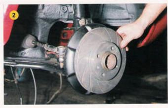
The standard front discs were replaced with grooved Black Diamond discs, designed to produce much better stopping power than the originals. There's certainly more metal in them though less ventilation. The manufacturers, claim that their brakes produce improved braking
