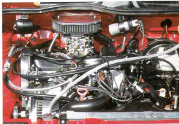
In the interests of reliability the engine now breathes through a Weber
