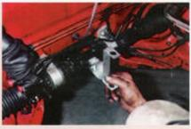
that the replacement bracket is precisely positioned. If you don't, the gearchange could be awkward to use and you may find that you need a fair amount of trial and error adjustment to be carried out, moving the bracket both from side-to-side and turning it in the vertical plane.
