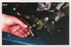
the pump bracket. It is most important that when you adjust the power steering belt, that the locknut on the inside of the brackets is released before the adjuster bolt is turned, and that the locknut is relightened after adjustment.
