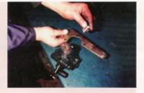
socket with an extension on it - or a pair of very long fingers if you have them! The other end of the bracket is then boiled in place via a threaded hole in the block. As this probably won't have been used before, the thread may need running out with a tap. The fixed adjuster bracket is now boiled to the engine block and fitted over the outer face of the pump bracket.
