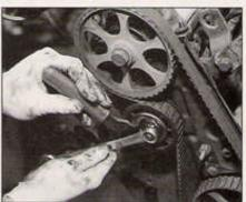
ABOVE LEFT, remove belt from the top down, working it loose from the cam sprocket first. Install the new tensioner hand tight.
